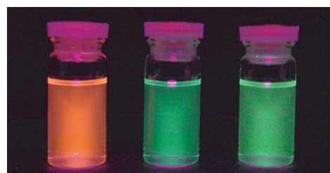
Figure 3. Photoluminescence from CdTe QD–silica nanoparticles in water under 365 nm UV excitation. The right sample is QD-S2, whereas the middle sample (lower TEOS concentration) is QD-S1 in Table 1. A sample prepared by using red-emitting CdTe QD (6 nm \phi ) is also shown in the left side.
